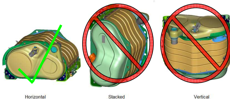
Figure 5.2 – 1206F aftertreatment mounting
