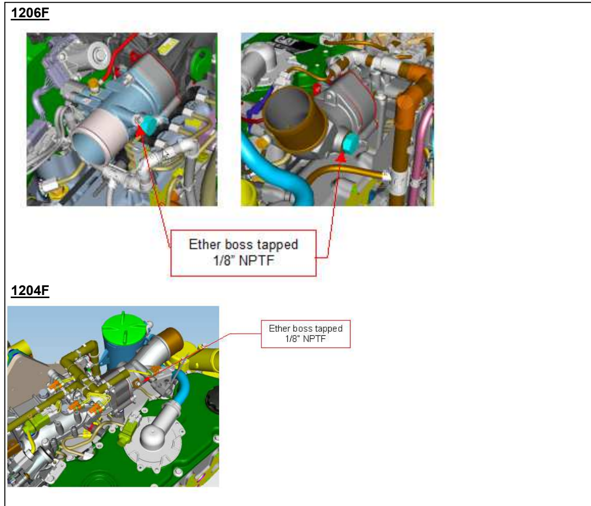
Fig 14.3 – Engine Boss' for Ether
