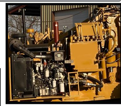
We upgraded this machine with a Perkins 1106D Diesel engine with 173 hp. All of the cylinders have been equipped with new seals. We replaced the old fuel tank with a new 79 gallon fuel tank. This ensures that the sediment from the old tank doesn't infiltrate the system. We replaced the old hoses and clamps to ensure proper presurization throughout this unit. Outfitted with a 390 Air Compressor mounted on the side of this machine adds a nice touch to this unit.
